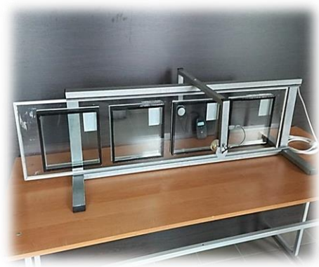
Fig. 4. General view of the laboratory stand for comparative studies of the permeability of visible flux rays for each type of double-glazed windows
